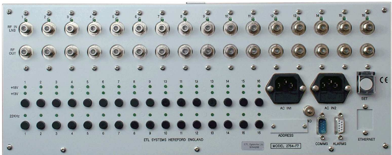
Rear View of Model 2764 with 75 ohm F-type connectors
